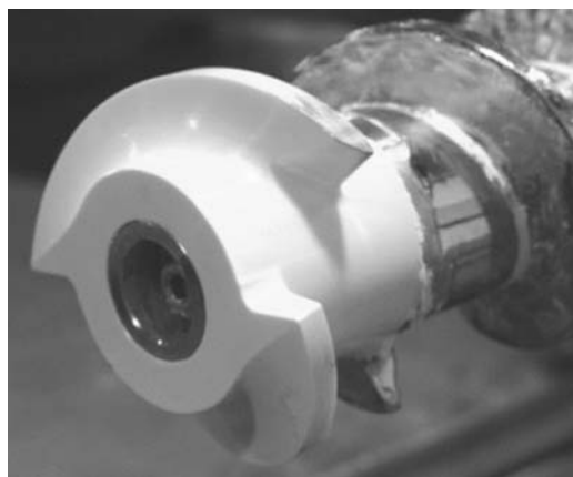
Fig. 6 Steel auger with \text{ZrO}_2 – front auger
