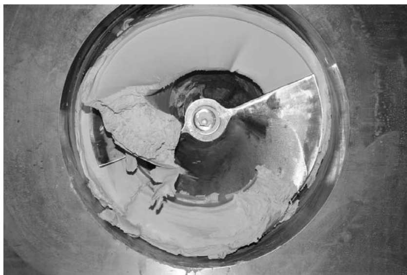
Fig. 9 Mass flow at the top auger
