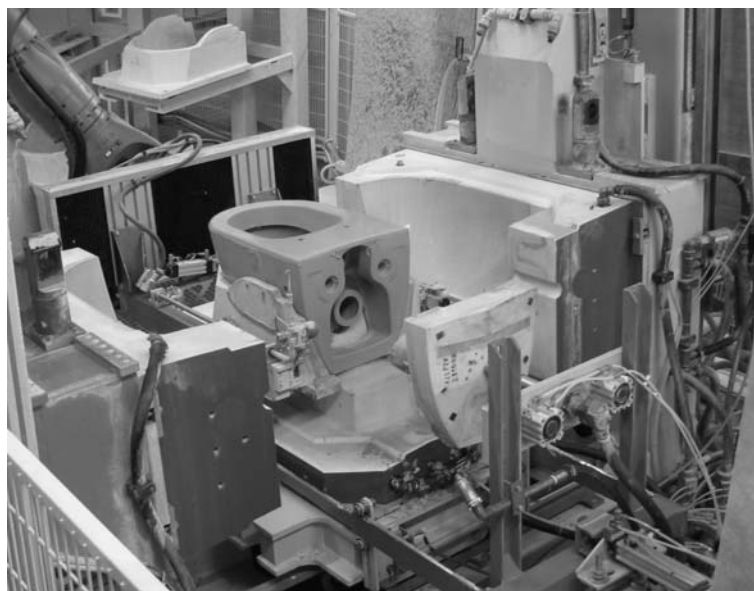
Fig. 14 High pressure casting machine
